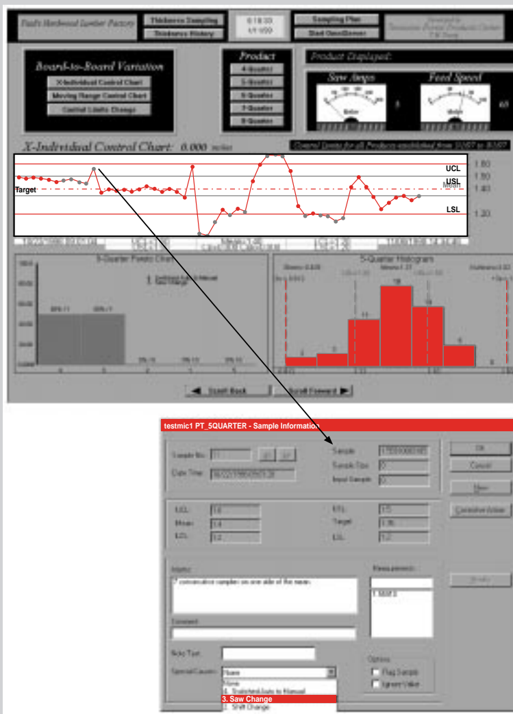
Figure 3. Wonderware®'s SPC HMI system as applied to hardwood sawmilling as part of the Tennessee Quality Lumber Initiative
