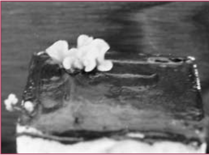
Decay fruiting bodies growing from L-joint field test sample.
