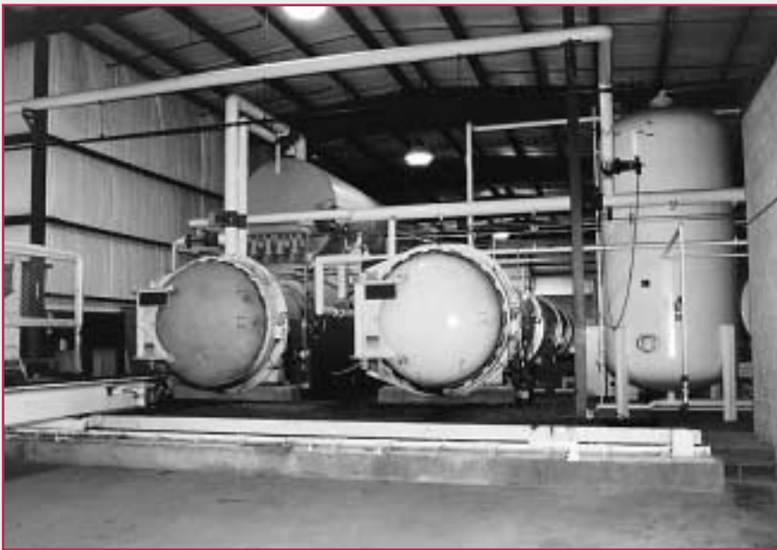
High-speed CCA treatment plant with accelerated fixation unit, northeastern United States.
