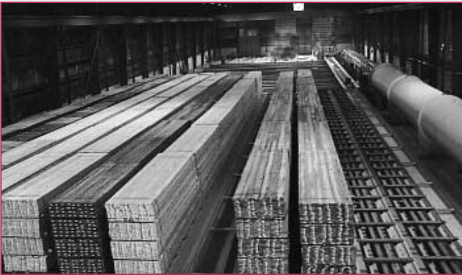
Figure 2. — High-capacity waterborne preservative southern yellow pine treatment plant with transfer deck. Plant capacity is up to 1 million board feet per day.
